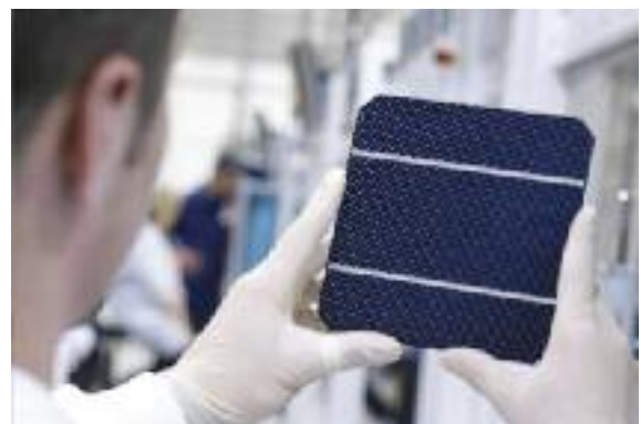
Monocrystalline solar cell.
